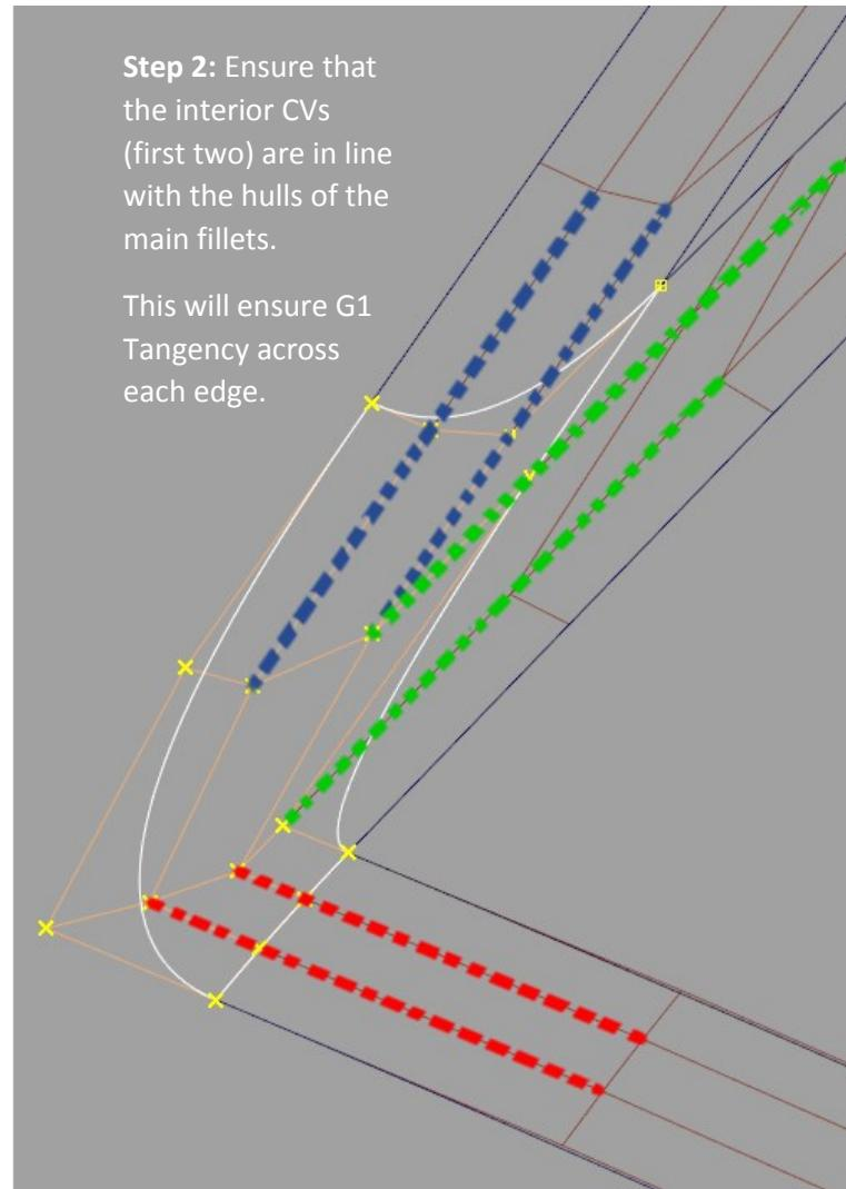
To display hulls only, without CVs, use Object Display > Control:
