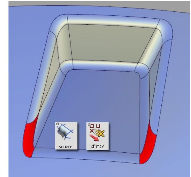
The key to success on all the corners is to align the CVs of the blend surface with the Hulls of the main fillet surfaces.
