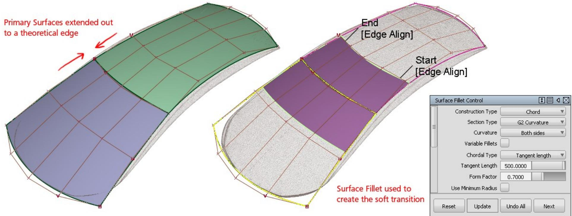
Creating a fillet on such a shallow edge can be tricky, and care needs to be taken to get a good relationship between the Primary Surfaces. Extra CVs will typically be needed to control the acceleration at the ends of the Primaries, as this has a strong influence on the behaviour of the Fillet.
